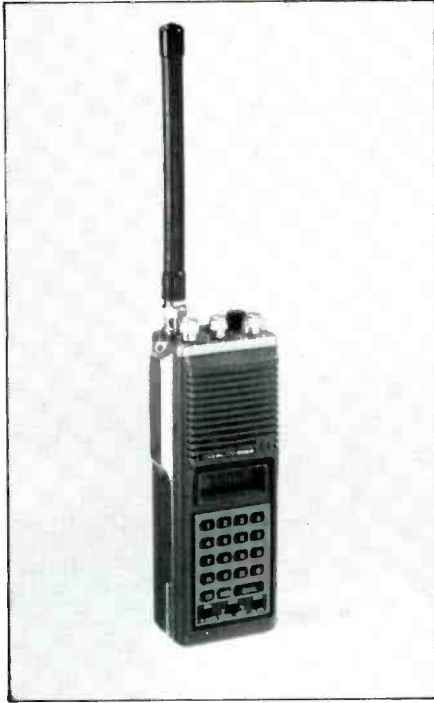
Keyboard programmable 2-meter FM ham transceivers such as these by Yaesu and Kenwood are more versatile and lightweight than standard military communications gear.
